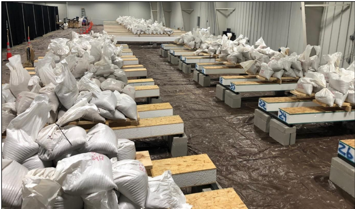
Fig. 2. Battery of full-scale matched SIP specimens undergoing the 90-day duration of load testing
