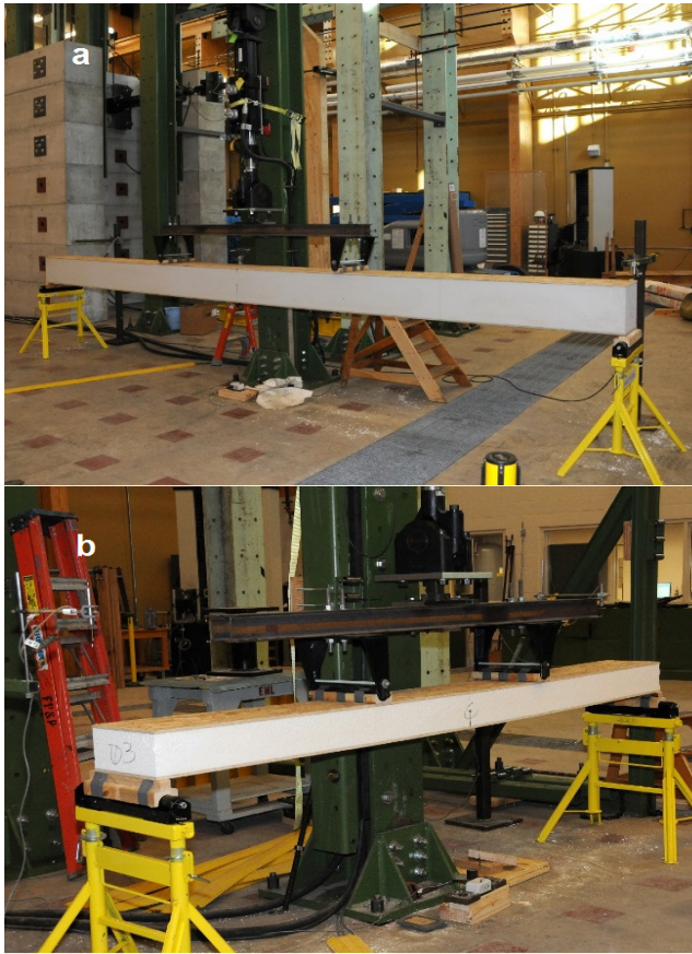
Figure 1. Static bending test setup: (a) 12.25-in.-deep specimens; (b) 6.5-in.-deep specimens.
