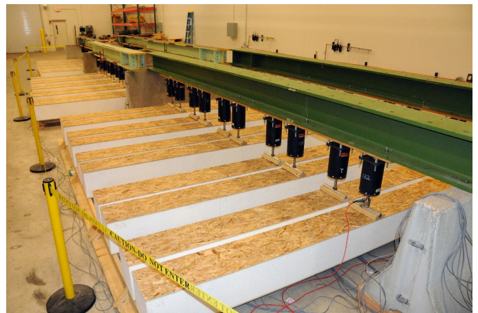
Figure 3. Creep test setup for the 12.25-in.-deep specimens.
