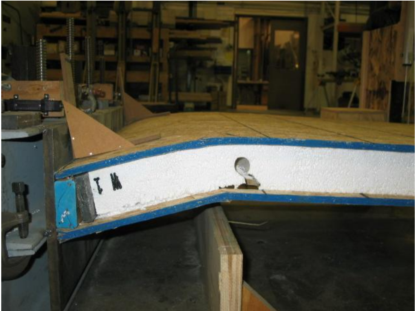
FIGURE C4. TYPICAL AXIAL LOAD (COMPRESSION) FAILURE (REPRESENTATIVE PICTURE)
