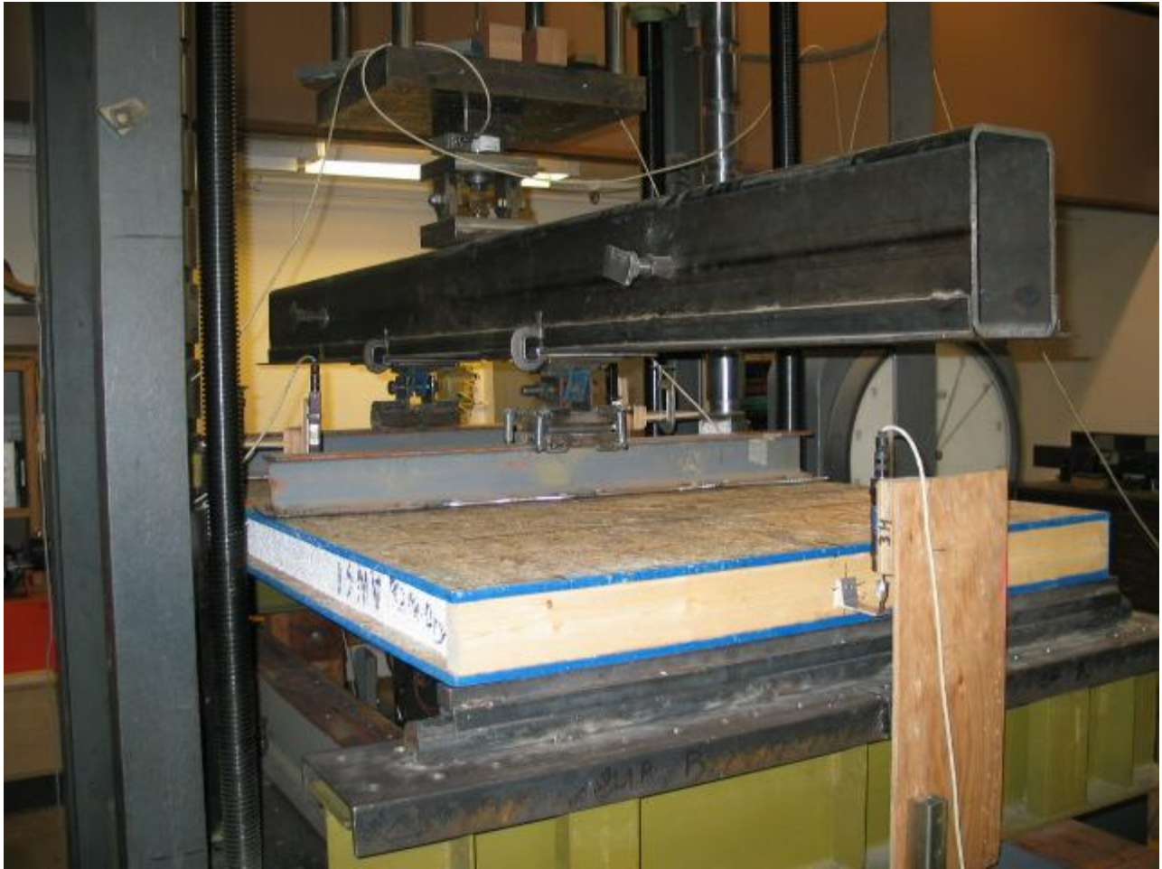
FIGURE C5. SIP IN TRANSVERSE LOAD TEST APPARATUS – THIRD-POINT LOADING APPARATUS
