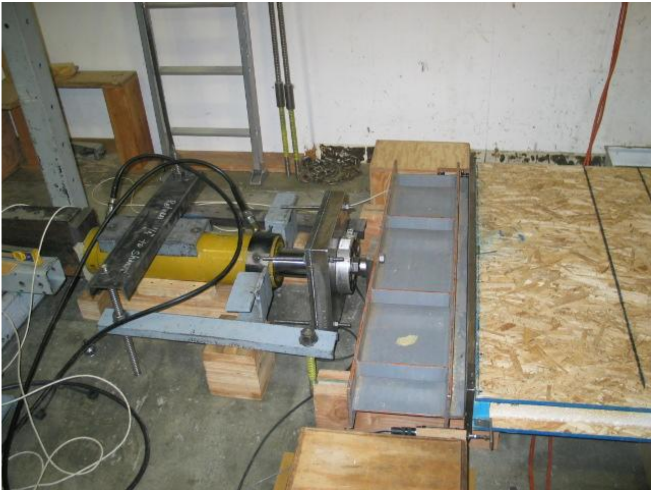
FIGURE C3. SIP IN AXIAL LOAD (COMPRESSION) TEST APPARATUS – LOAD HEAD END
