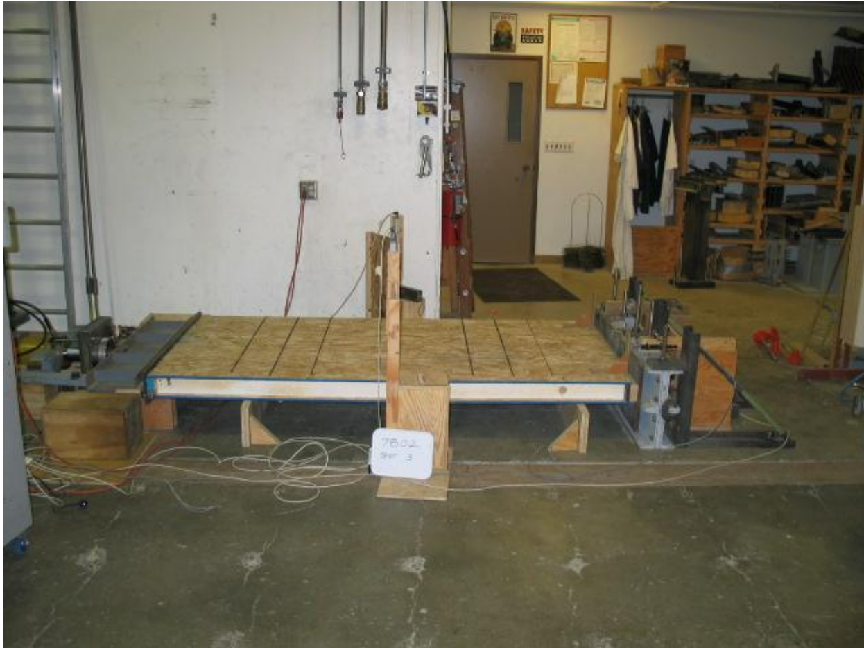
FIGURE C1. SIP IN AXIAL LOAD (COMPRESSION) TEST APPARATUS
