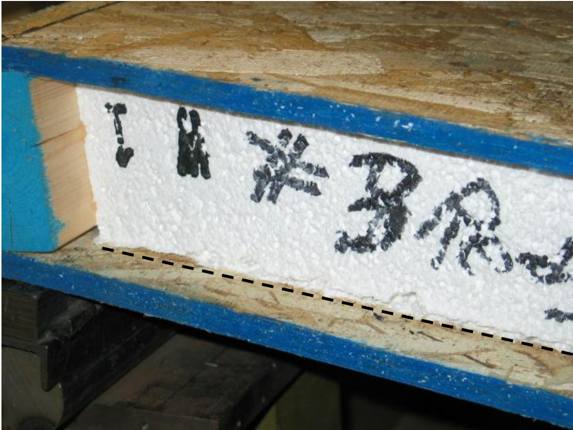
FIGURE C7. TYPICAL SIP TRANSVERSE LOAD FAILURE (Failure plane at the foam core and OSB facer interface shown just above dotted line)
