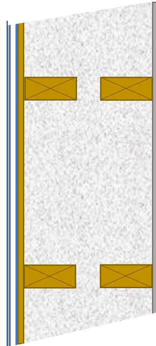
Double-Wall Framing 10% F.F.
