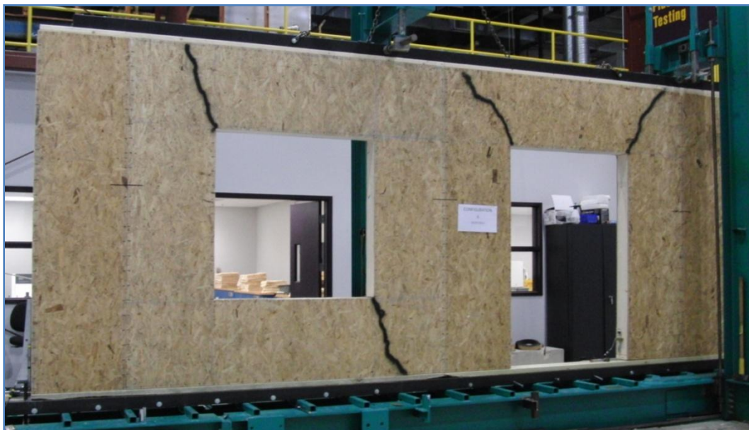
Figure 12. Configuration 6 Cracking of OSB Skins (black lines indicate location of cracks)
