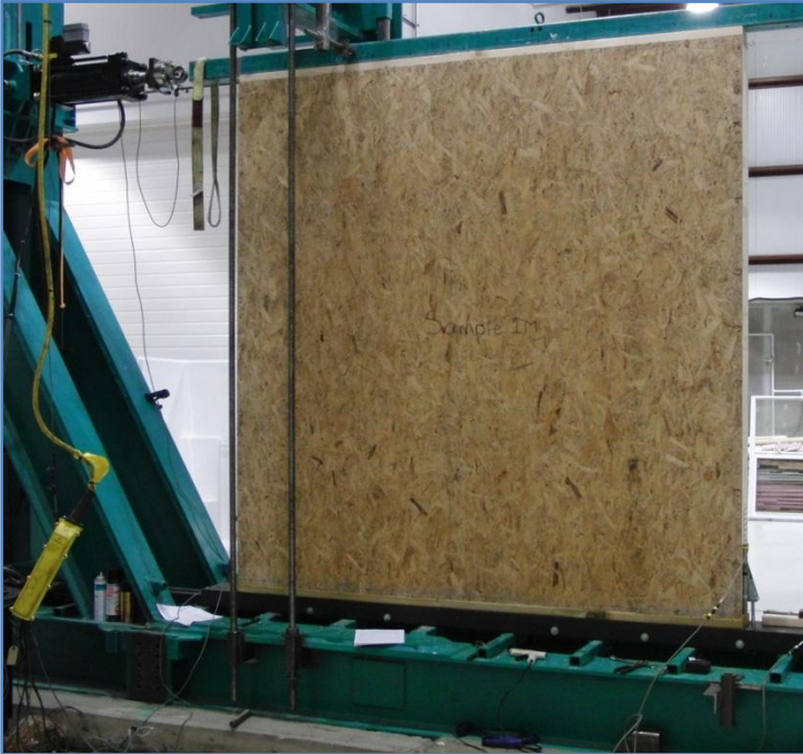
Figure 2. Shear Wall Specimen (Configuration 1M)
